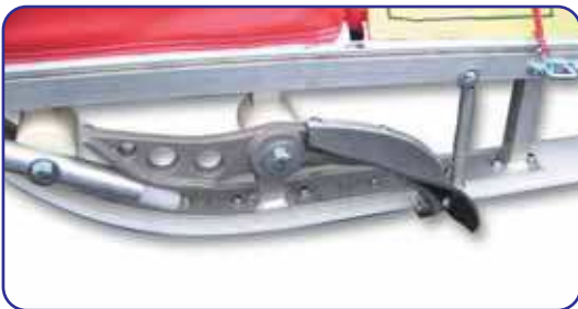
Brakes on copper bearing with splash-proof skirt
